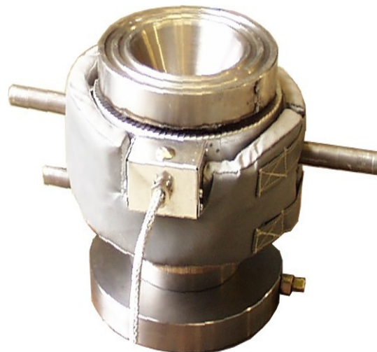
Figure 5 : Experimental device using a conical die The bulge device consists of two chambers that can be used if necessary as pressure and/or counter pressure chambers. The pressure and/or counter pressure inlet and outlet take place through a drilling in the cylindrical and/or
